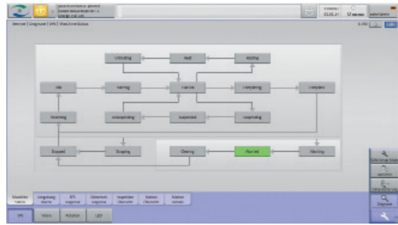
Seidenader uses PackML as an internal standard applied universally by all programmers, which makes the software easier to understand, diagnose and operate.
