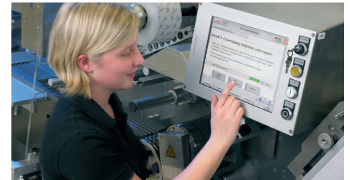
The operator console for the CP600 blister machine is based on a decentralized Automation Panel, which B&R modified according to Mediseal’s design requirements to fit directly into the console housing.
