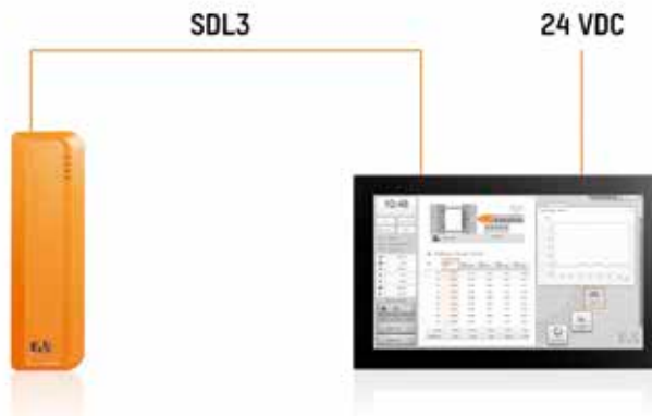
If 24 VDC is already being supplied, the Automation Panel can be connected directly to the Automation PC 910 via SDL3.
