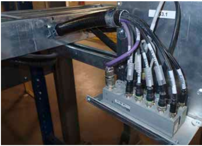
A flexible IP67 rated machine-mount I/O system with 16 programmable channels was implemented for conveyor line control, allowing each channel to be individually assigned as a digital input, digital output or high-speed counter.
