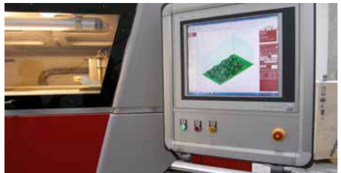
The operator terminal of the new VX2000 from voxeljet, based on a touch-screen Power Panel from B&R. The HMI application runs on the same PC that prepares the print data for the 3D printer.
