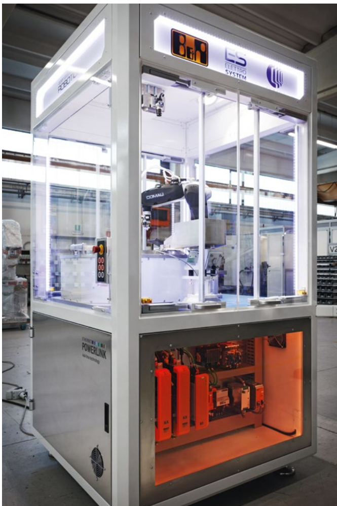
With industries demanding ever more compact manufacturing equipment, reducing the number, size and complexity of automation components becomes an important design challenge. The COMAU control cabinet solves this challenge with advanced B&R products like the ACOPUS P3.
