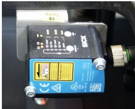
Smart and well-connected: the DT35-B15251 distance sensor from Sick does more than just measure. With IO-Link, it opens up exciting possibilities for IIoT manufacturing.
