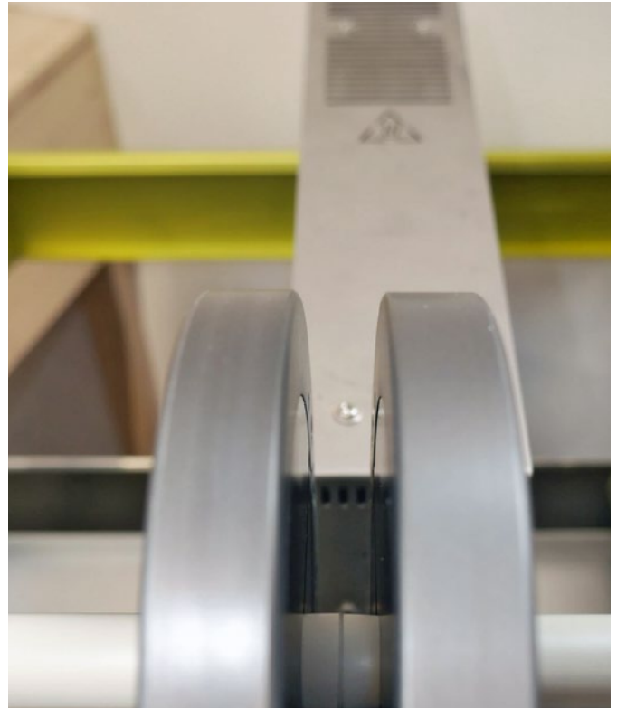
A bead of molten polypropylene joins two pieces of butt-fused 20-millimeter pipe clamped in place on the machine.
