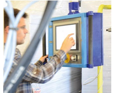
Since the retrofit, the trimmer is easy and intuitive to operate via the new touchscreen.
