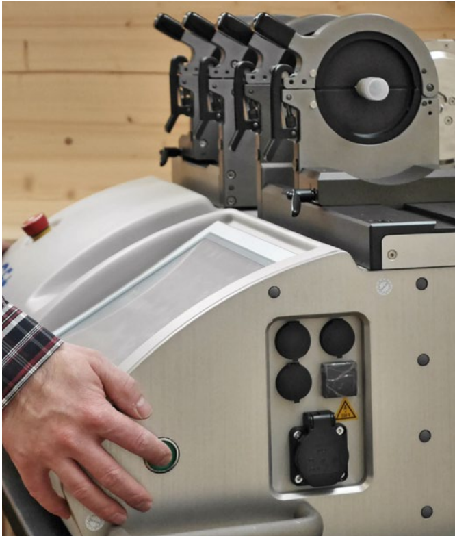
A machine operator executes a movement using two-hand operation (green button). The buttons for two-hand operation are connected to and evaluated by a B&R safety controller.
