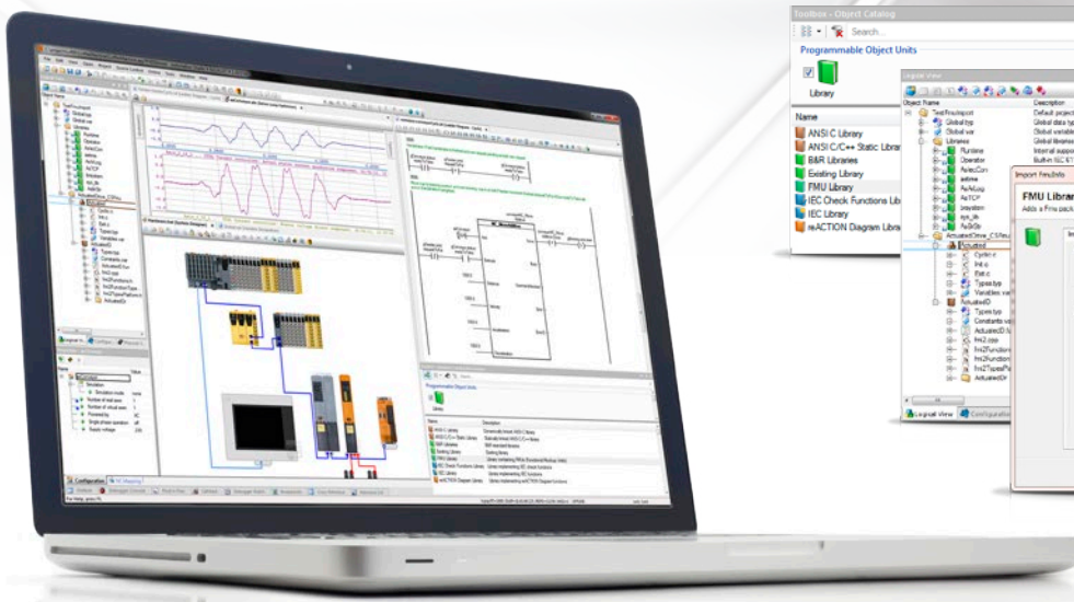
Dragging and dropping Functional Mockup Units (FMUs) into Automation Studio opens a convenient import wizard. Updating previously imported FMUs is even easier.
